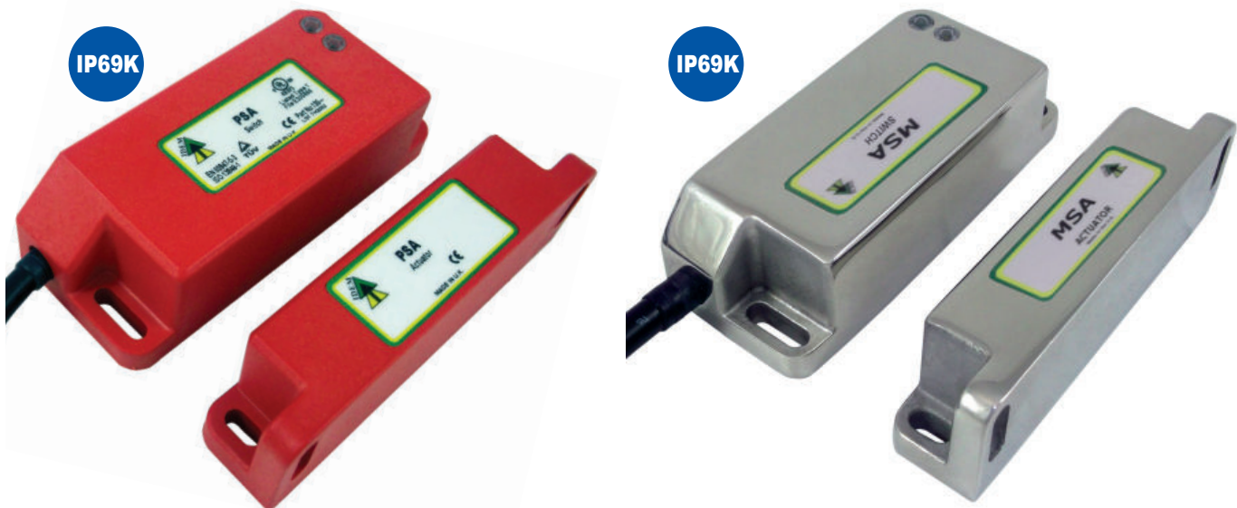
Tested to ingress protection degree IP69K (high pressure hosing with detergent at 80C and 100psi)
