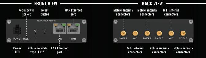
Mobile signal strenght LED\* RED color when signal RSSI is between -110 and -82 dBm, YELLOW color when signal RSSI is between -82 and -52 dBm, GREEN color when signal RSSI is more than -51 dBm Mobile network type LED\* YELLOW color when device is connected to a 3G network, GREEN color when device is connected to a 4G notwork, BLUE color when device is connected to a 5G network.
