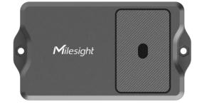
EM400-TLD is a distance sensor based on ToF (time of flight), which is mainly used for detecting the fill level and position status. With an appropriate FOV with the maximum field angle of 27°, it has almost no blind spot when installed on small-sized waste bins or containers. The embedded temperature sensor enables it to monitor whether the containers are burning for security reasons.
