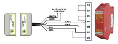
One switch connected to an SCR-2 or SCR-3 to give Dual Channel guard monitoring but with Automatic Start.
